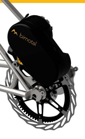
**Innovative** | mounts to the same points as your externally mounted disc-brakes
