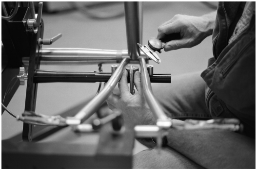
Titanium requires careful handling, and Potts meticulously measures, machines and cleans the tubing for each frame.
