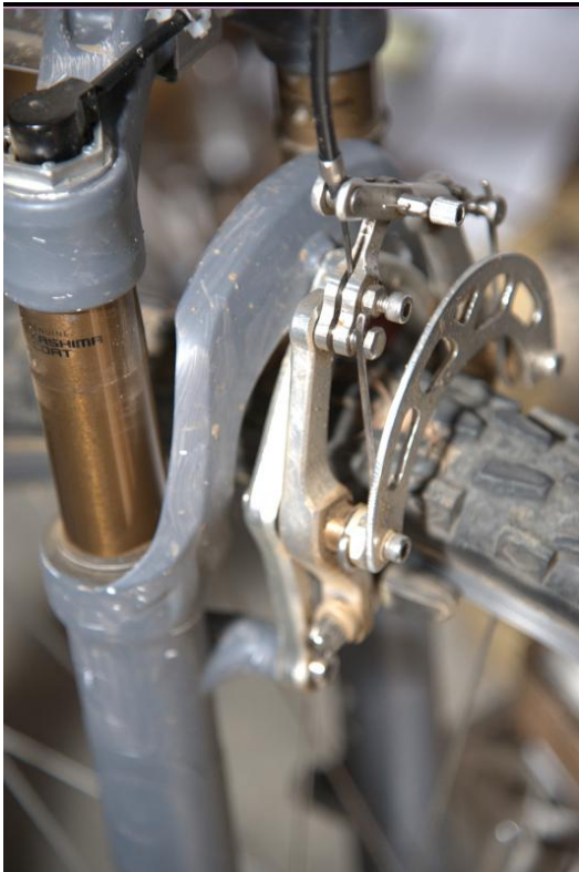
Cunningham designed and hand-machined the many small parts for the brakes on the DIA bike.
