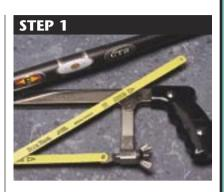
arbon tubing (i.e. handlebars, seatpost, fork steerer tubes, etc.) can be quite easily cut using a standard hacksaw. There are, however, some precautions that must be taken to prevent damage to the component, and harm to yourself.
