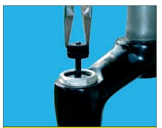
5. Remove the adjustment unit with the pliers.
