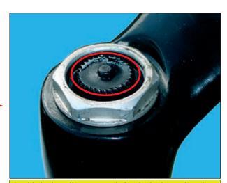
4. This is the adjustment unit for the lock-out function.
