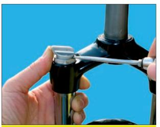
3. ... a slot screwdriver as lever, taking care not to scratch the top cap.
