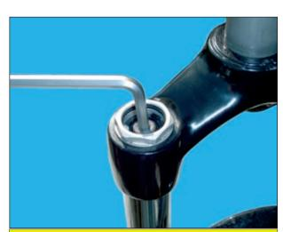
6. Now, please check if the lock-out cartridge is fastened, using the 5mm Allen key. If not, then tighten.
