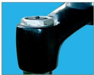
9. Re-insert the adjustment unit (toothed washer with short 4mm Allen key) and take care to push it well into the top cap, until it is flush with it. Else, the Allen key is not inserted properly and the lock-out will not work.
