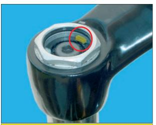
8. No matter which of the two above mentioned claims are present, please turn the 4mm Allen key clockwise, until you feel the stop. Now, please remark the position of the "yellow" marked stopper ( which is actually black), before re-inserting the adjustment unit.
