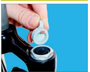
10. Now, keep in mind that the fork is in locked condition. Please remark the "red" marked stopper on the lock-out knob. This stopper has to be inserted to the left of the stopper in the top cap.
