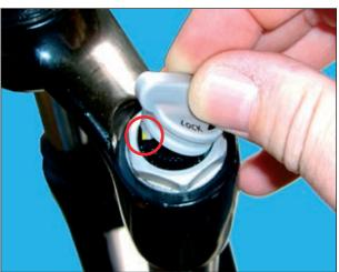
11. If you consider the stopper (yellow) in the top cap to be placed in the position of 12 o'clock, then you have to place the stopper of the knob at 11 o'clock. Now turn the knob counter-clockwise and check if the fork is un-locked.
