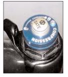
21. Insert compression damper top cap seal (o-ring) over top cap (fig 21a). Place compression knob onto top cap, with dial at 3 o'clock position. The Remote knob should also be positioned with cable set-screw at 3 o'clock (fig 22b). Using snap ring pliers, secure compression knob with external retaining ring (fig 21c). Insert gate adjuster cover cap (fig 21d).
