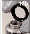
**13.** Using a long dowel, push rebound damper seal head up through the upper tube.
