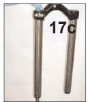
**18.** With rebound damper shaft in the fully extended position, measure and pour 95cc (+/-5cc) of RockShox 5wt suspension oil into upper tube, through crown (fig 18a).
