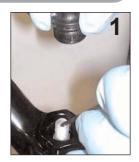
2. Gently pull external rebound adjuster knob and remove from right shaft bolt. (11.4308.846.000, 05 External Rebound Adjuster Knob, Short)
