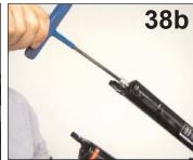
39. Insert external rebound damper knob into damper shaft bolt. Push in to secure.
