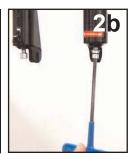
4. Using a plastic mallet, tap both shaft bolts free. This frees the shaft ends from the lower leg shaft bore press-fit, and allows the lower leg assembly to be removed from the upper tubes (fig 4a and 4b). Using the 5mm hex wrench, or your fingers, remove the shaft bolts from both threaded shaft ends (fig 4c).
