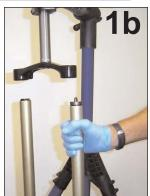
2. Clamp right (damper side) upper tube into bicycle stand. Using a 5mm hex wrench, loosen right shaft bolt 2 to 3 turns. Do not remove shaft bolt completely. (fig 2a) Tap shaft bolt free using a plastic mallet. This frees the damper shaft press-fit from the inner shaft bore inside bottom of lower leg. (fig 2b)
