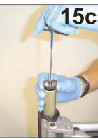
NOTE: INSERT A LONG PLASTIC OR WOODEN DOWEL INTO THE UPPER TUBE TO KEEP REBOUND DAMPER IN FULLY EXTENDED POSITON. THIS HELPS WHEN TIGHTENING THE SHAFT BOLT. (FIG 20c)
