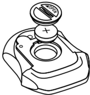
FIGURE 18: BATTERY INSTALLATION
