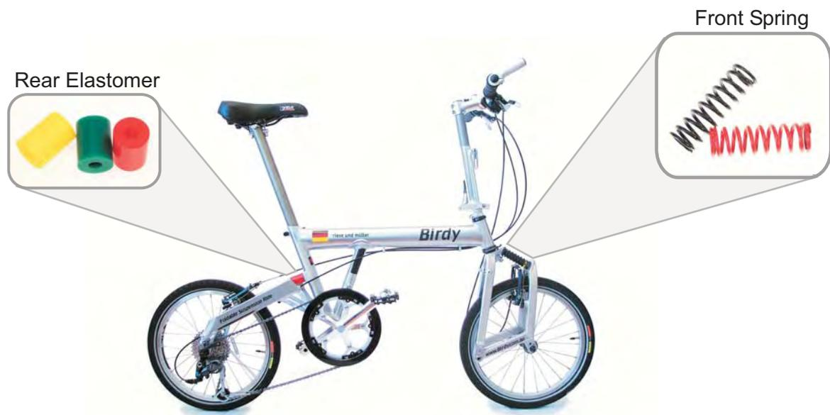
**1.** One of the unique features of the Birdy is the integration of the folding joints with the suspension. By using the pivot points of the rear and front swingarms for both folding and suspension, the designers have achieved a jointless frame which is very stiff, stable and light. (A folding joint in the frame which is used on many other folding bikes is a weak point and makes the bike heavier and more fragile).
