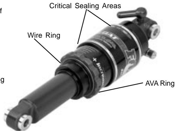
Air sleeve service can be performed as on other FLOAT shocks. Clean AVA seals after every other normal FLOAT seal service, especially if riding conditions are muddy or dusty. Carefully remove wire rings and air sleeves. Clean and inspect seals and parts for damage or wear. Re-lubricate and carefully re-assemble. Refer to diagram for areas with critical sealing and lubrication needs.
