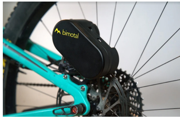
The Elevate motor quick-connects to brake mount studs
