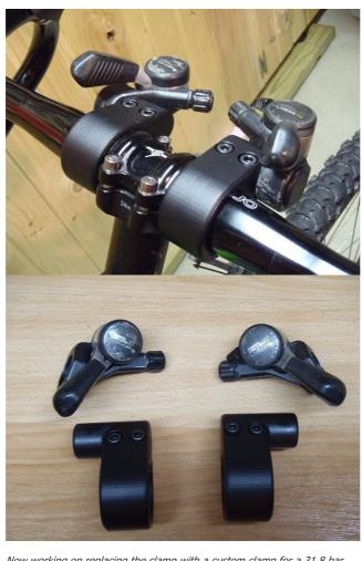
Now working on replacing the clamp with a custom clamp for a 31.8 bar.
