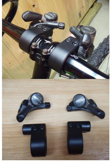
Now working on replacing the clamp with a custom clamp for a 31.8 bar.
