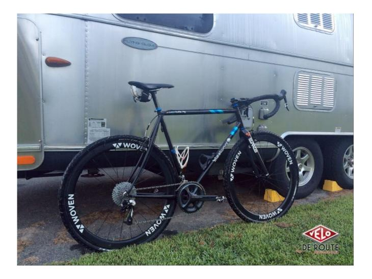
I raced this bike a few times with these Bontrager 700c x 38mm tires, notably, at Vermont Overland. They measured closer to 40mm, and felt good at speed, as this bike has 70mm bottom bracket drop. Rlm brakes made it impossible to run 650bs.
