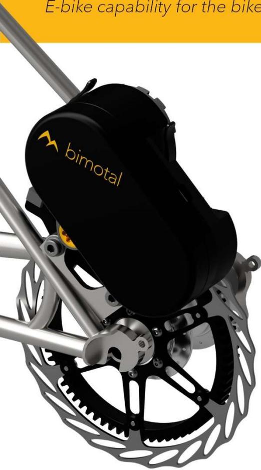
**Innovative** | mounts to the same points as your externally mounted disc-brakes
