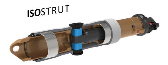
The fact that there's no link to drive the IsoStrut shock is what sets it apart from a typical rear suspension design. Everything is built into a carbon fiber carriage which moves on 36mm bushings, and the shock is connected via hardware that runs through the center of that carriage, along with slide bushings that also prevent any rotation.
