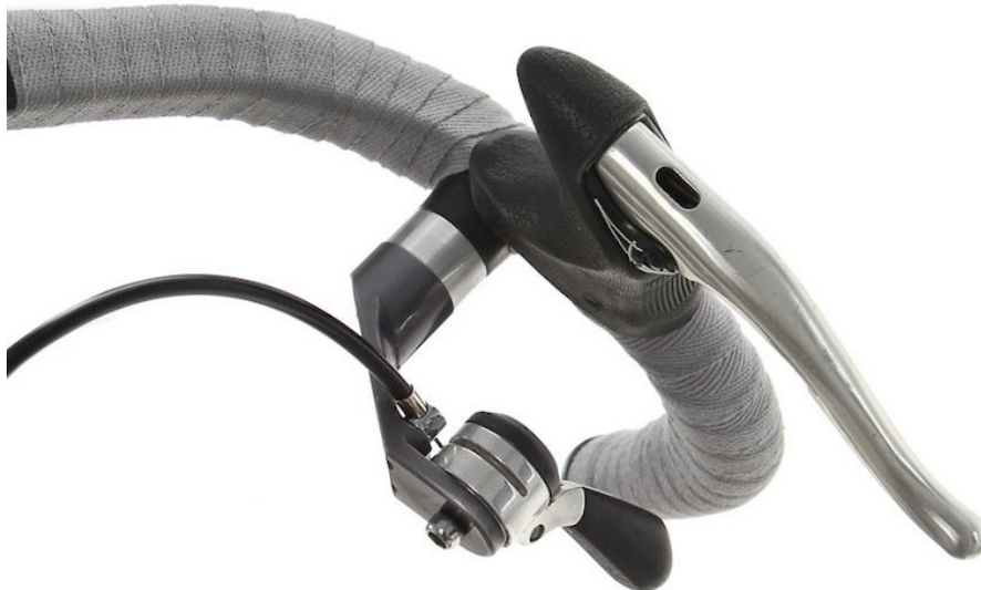
Crude, but effective. Charlie's adapters put the thumb shifters within reach while the rider was in the drops. - Pro's Closet photo
