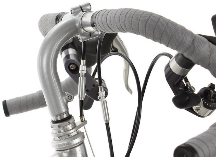
Charlie brazed an extension tube that protruded above the fork's threaded steerer, where his clamp-on stem attached. - Pro's Closet photo
