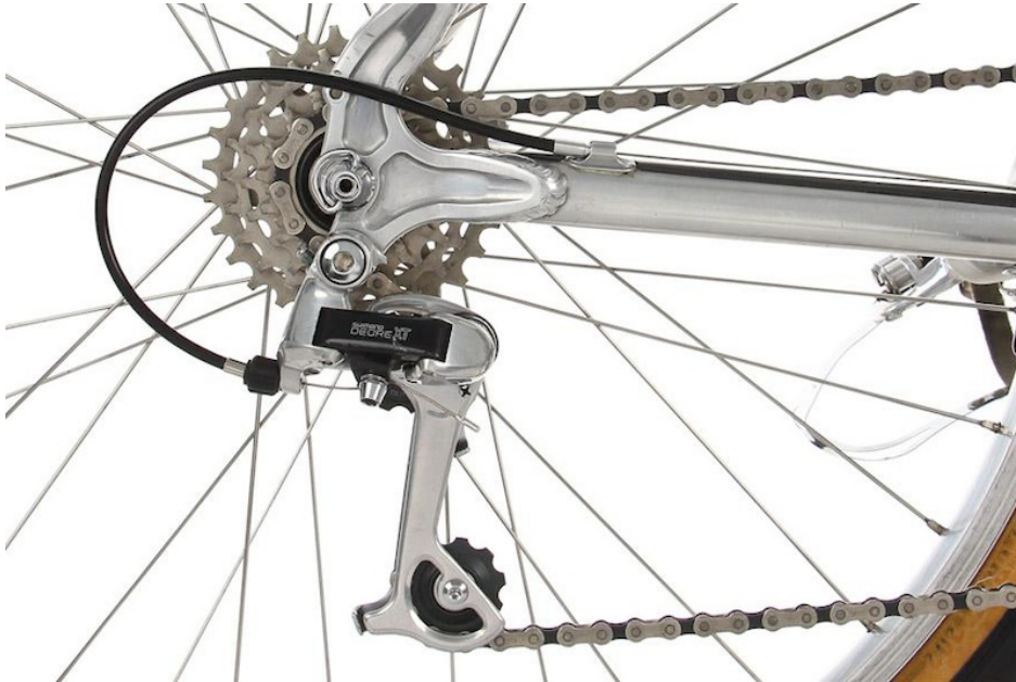
Gearing was limited in 1988. This bike has a conventional three by crankset. At the time, Charlie was making wide ratio seven-speed cogsets. - Pros Closet photo
