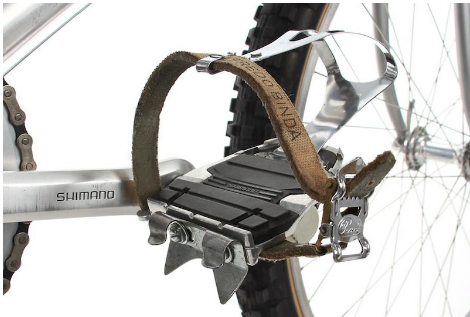
Perhaps his simplest invention, "Toe Flips" screwed onto the back of the pedals for quick entry. Thousands were sold. - Pros Closet photo
